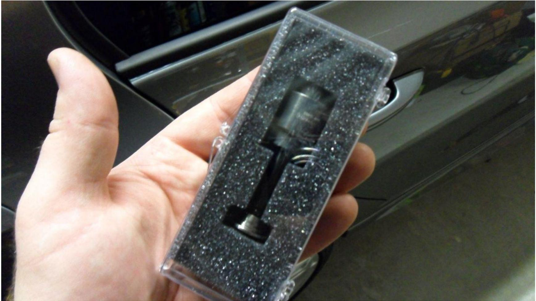
19) Ensure the Autotech piston (notice the thickness difference from the OEM piston) is clean and free of contaminants by dipping it in petrol before inserting it into the stainless seal holder. Insert it from below (the threaded end of the stainless steel seal holder) as shown by the arrows in the pic below.
