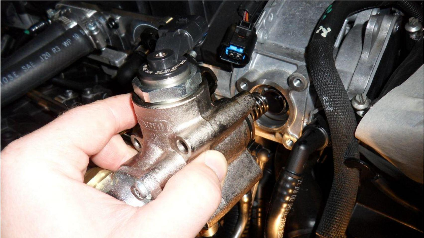
12) With the pump removed, you will have access to pull out the cam follower and inspect the level if wear on it. In my cars case, the 10,000km its travelled has not created any wear to worry about on the cam follower.
