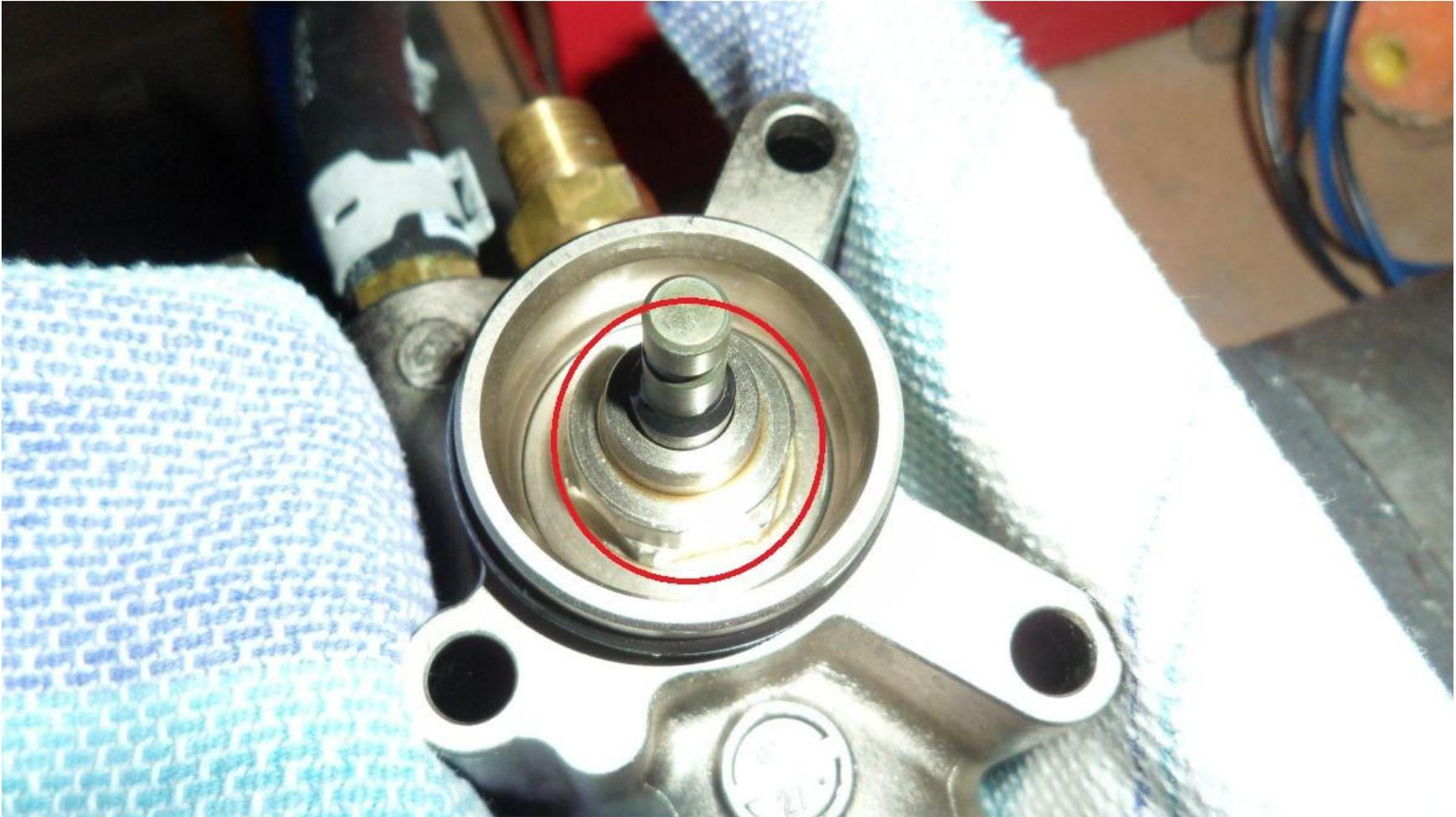
23) Now clean the spring you removed earlier by dipping it in petrol. Lift the piston up as far as you can out of the HPFP body. Click the spring back in place over the top of the piston.
