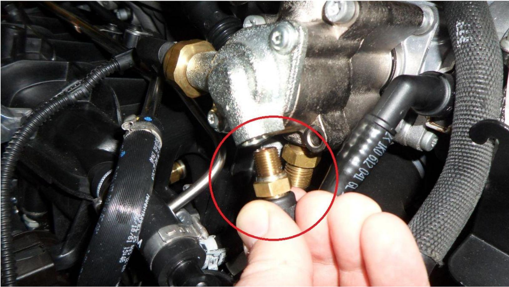
7) Using a 17mm spanner, crack and undo the silver high pressure fuel line leading into the bottom of the HPFP. Undo the nut completely and slide it back out of the way.
