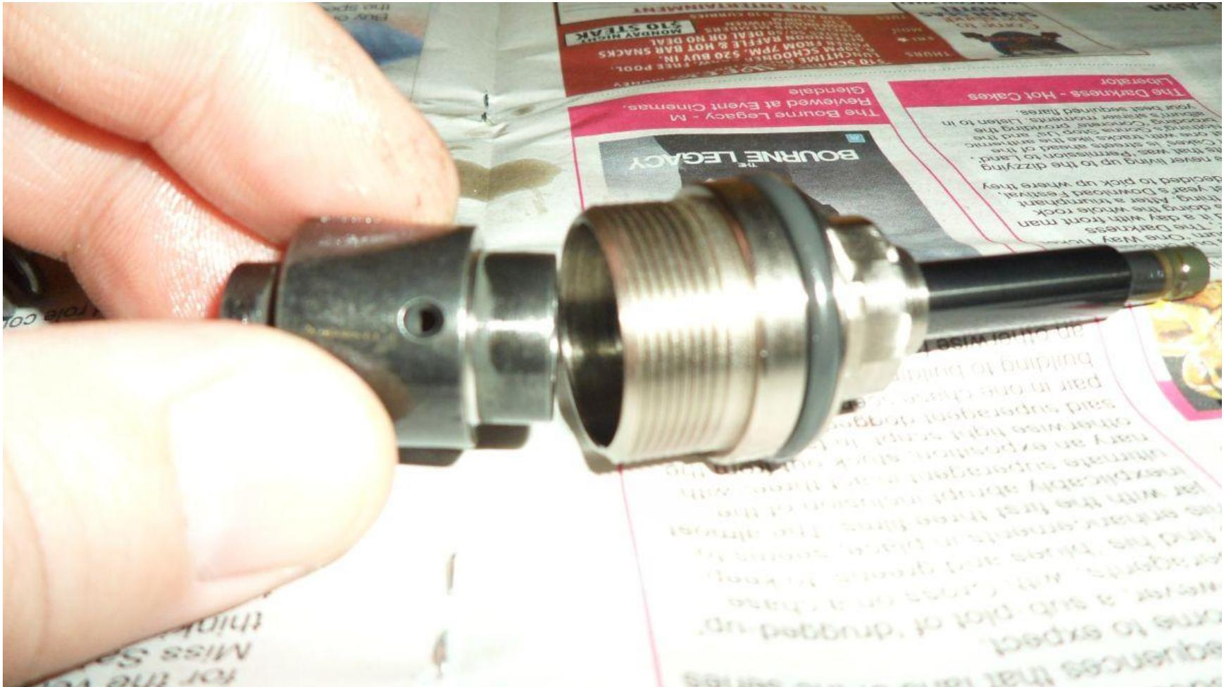
21) We will now put these parts back into the HPFP body. Lubricate the rubber seal on the stainless steel seal holder with some clean engine oil. Just use your finger to rub the oil onto the seal. Insert the parts back into the HPFP body.
