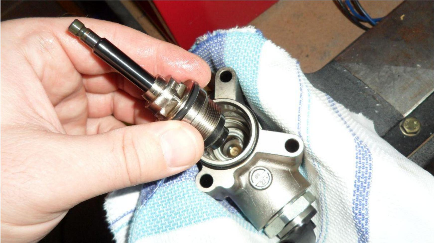
22) Clean the 18mm nut you removed earlier and also clean the 18mm long socket you are about to use to tighten the nut up (this is to ensure no pieces of dirt fall into the HPFP during re-assembly). Tighten the 18mm nut up
