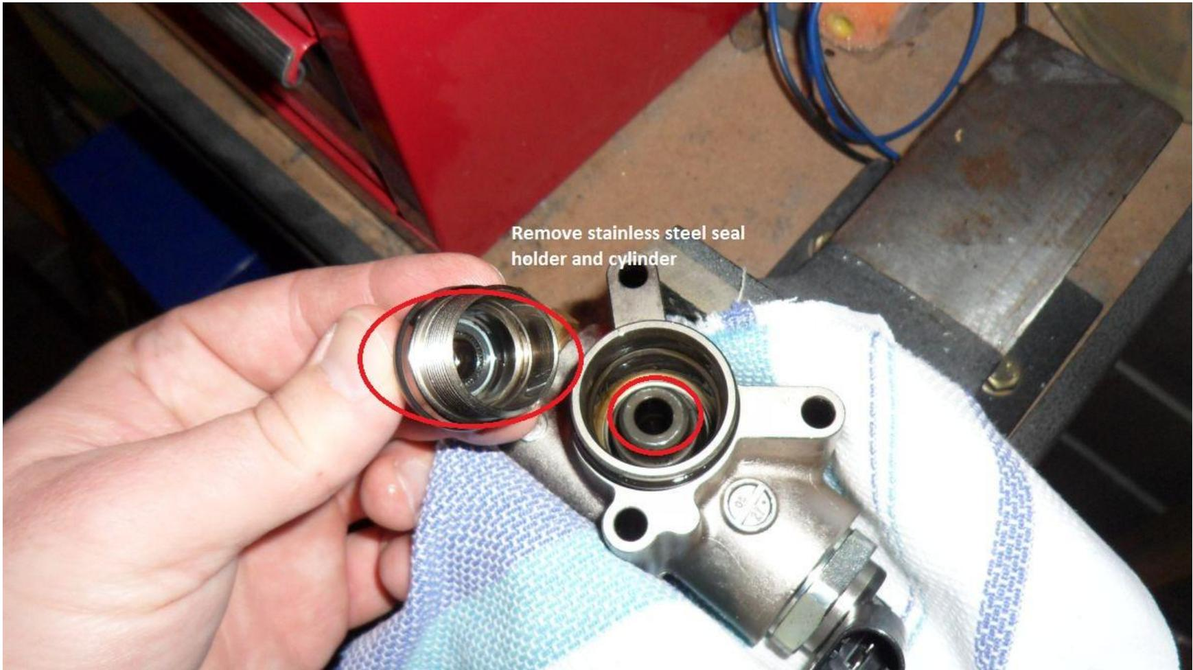
17) You should now have the following items removed from the HPFP. The only parts we are going to re-use are the stainless steel seal holder and the spring.
