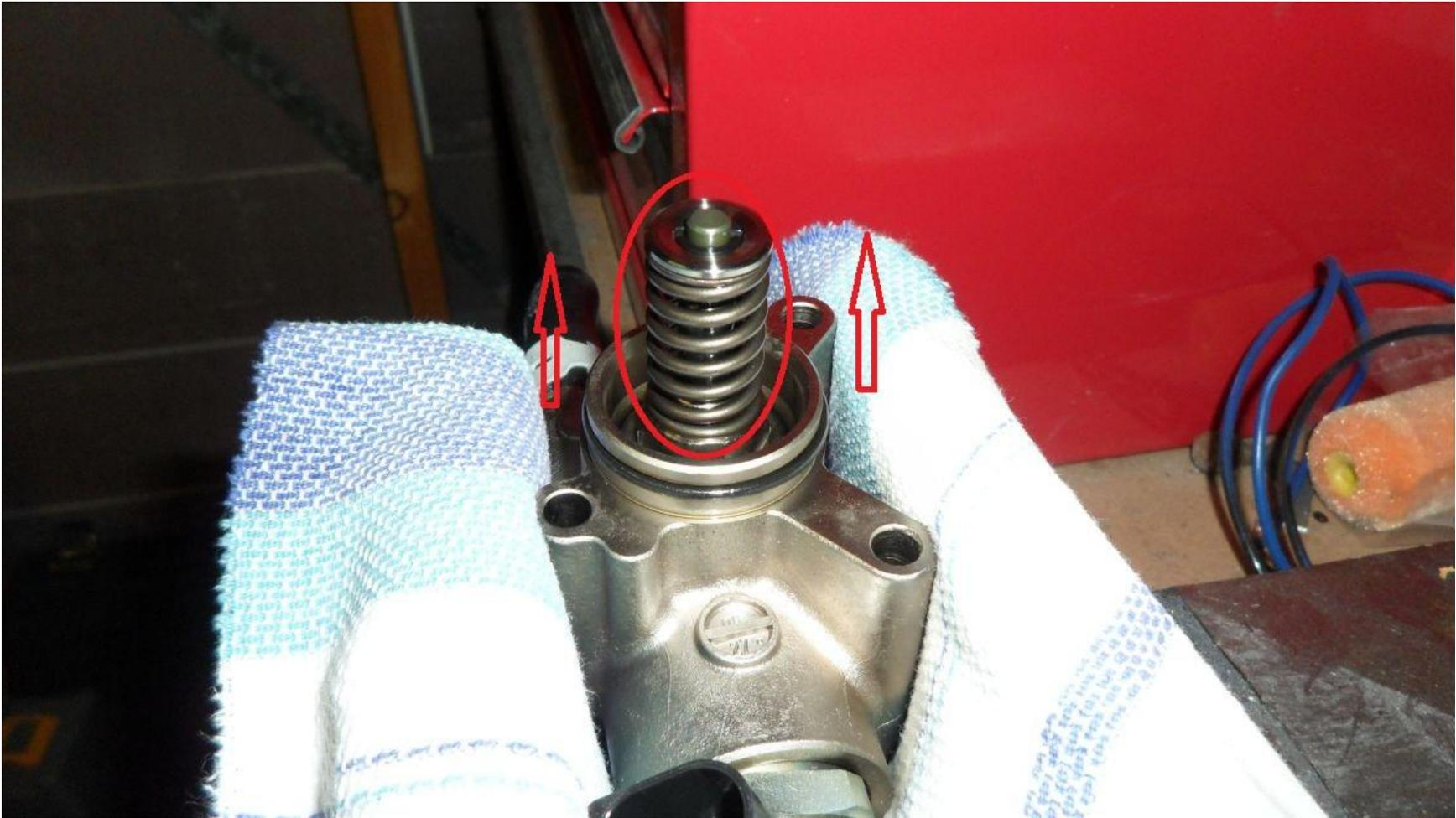
15) With the spring and piston removed, you have access to the 18mm nut which needs to be removed. You can do this with a standard 18mm socket now, but you will need a long 18mm socket to put it back on later.
