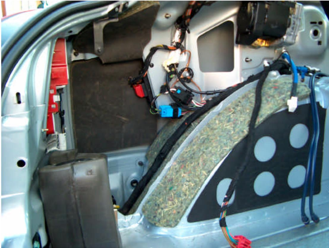
The AMSS is slightly larger than the original so some of the obstacles in the rear wing need to be tidied up before the unit will fit properly. Firstly unclip the wiring loom running down the seam along the wheelarch. This needs to be pushed toward the back of the rear wing cavity. Using an 8mm spanner or socket, unscrew the nut holding the earth straps to the chassis.
